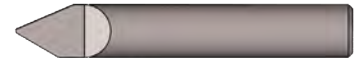
Engraving Tools Engraving Tools come in a large variety of angles and sizes. These solid carbide tools will engrave on a large variety of materials. The tool tip is held to \pm 0.001 inch tolerance for uniformity.
