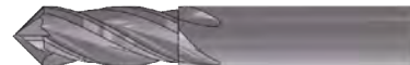
Drill Mills Drill Mills are designed for milling, chamfering, and light spotting applications. They come with two or four helical flutes each offered in included angles of 90 or 120 degrees. The cutter diameter sizes range from 1/8" to 1/2".
