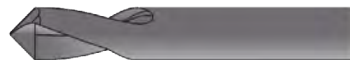
Spotting Drills Spotting drills are a valuable first step in the holemaking process. The tool is solid carbide with a precise point angle that is held to a one-degree tolerance for true centering. It is available in 82, 90, 100, 120 and 142 degree point angles.
